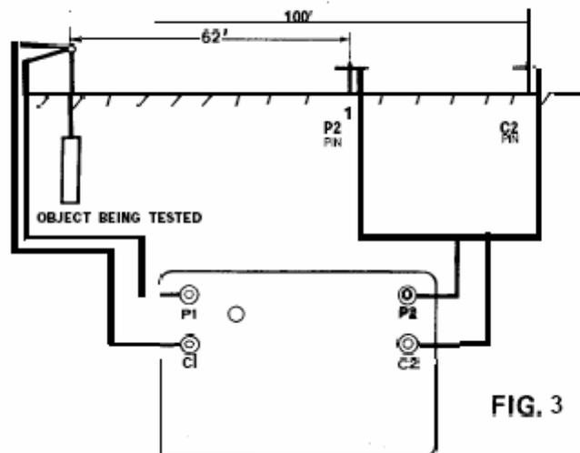
Normally 100 feet would be typical for a ground rod 15 to 20 feet deep. Connect "P2" to a pin 62% of distance from the object being tested to the "C2" Balance and read in usual way. Fig 3
